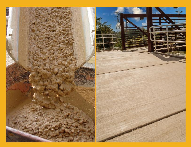
**SikaColor®-120 G Granular Integral Concrete Colorant** is free-flowing concentrated pigment granules designed to permanently color concrete and other cementitious materials. It can be poured directly into concrete mixes, conveyed by gravity feed or pneumatic equipment, or pre-dispensed into repulpable bags.
