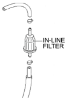
Figure 16. In-Line Fuel Filter
