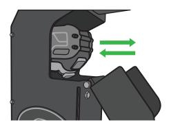
Check all linkage for proper activation of drill trigger.
