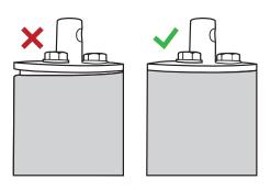
Verify the pipe insert is installed properly and not at an angle.
