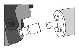
After the tube has been attached to both handles, install the battery. With both operators holding firmly on the handles lightly pull the variable speed trigger to see which direction the pipe turns. The pipe should roll away from the operators for proper operation. If the pipe rolls towards the operators, simply change the rotation of the pipe by pushing the directional button on the side of the machine.
